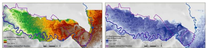
*Left:* LiDAR derived Digital Terrain Model (DTM) of Congaree River floodplain. *Right:* HEC-RAS derived flood inundation model of Congaree River floodplain.
